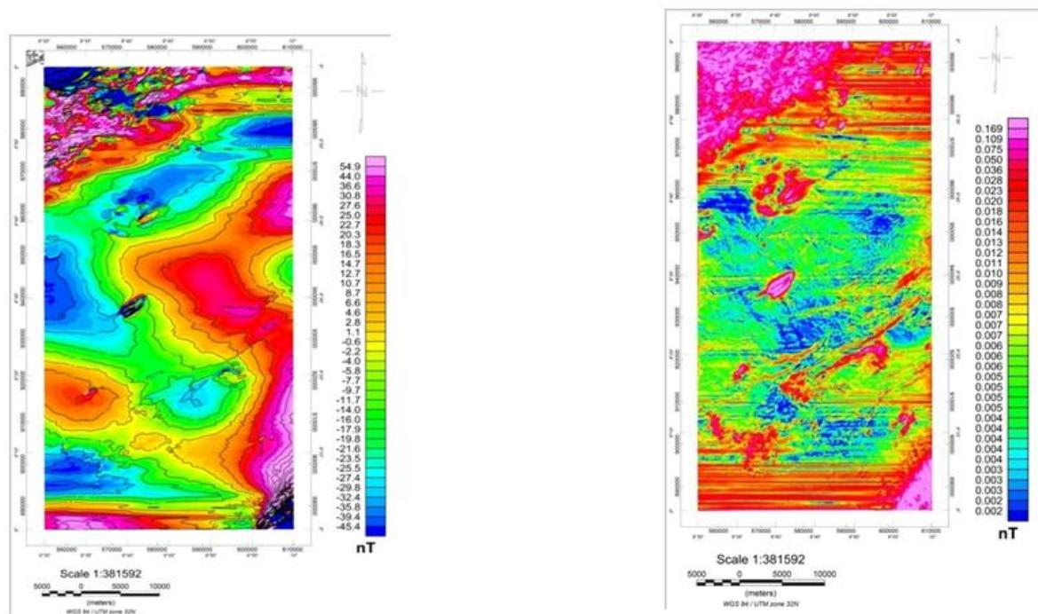
**Fig.5.** Residual map with contour **Fig .6.**analytical signal of the area
